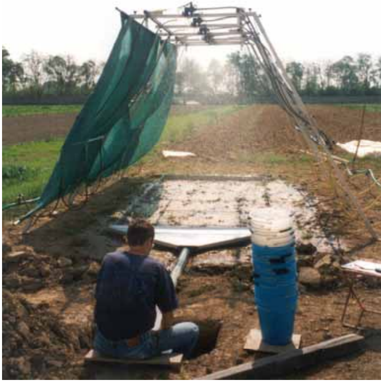
Fig. 1. The rainfall simulator at work
